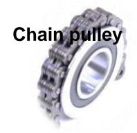
Chain pulley's get as well used at machinery and forklift trucks. The pull chains are turned around the chain rollers, which are fixed on the lifting cylinder or internal mast. Depending on the lifting gear construction, the wrap-around may be up to 180°. The requirements for the rollers depends on the number of the chains, the wrap-around angle as well as the load capacity of the machine.
