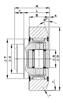
Combined bearings adjustable by eccentric bolt for I-Profiles
