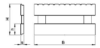
Fork carrier frames will be fitted to rapid, tensioning attachments to facilitate an integrated side slider or for attaching extension devices as required.
