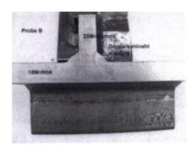
**Figure 2:** Profile of 25MnV5mod and 18MnNb6 single-layered, double-fillet welds
